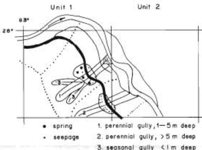
Fig. 23.17 The drainage and hydrogeological attribute zones
