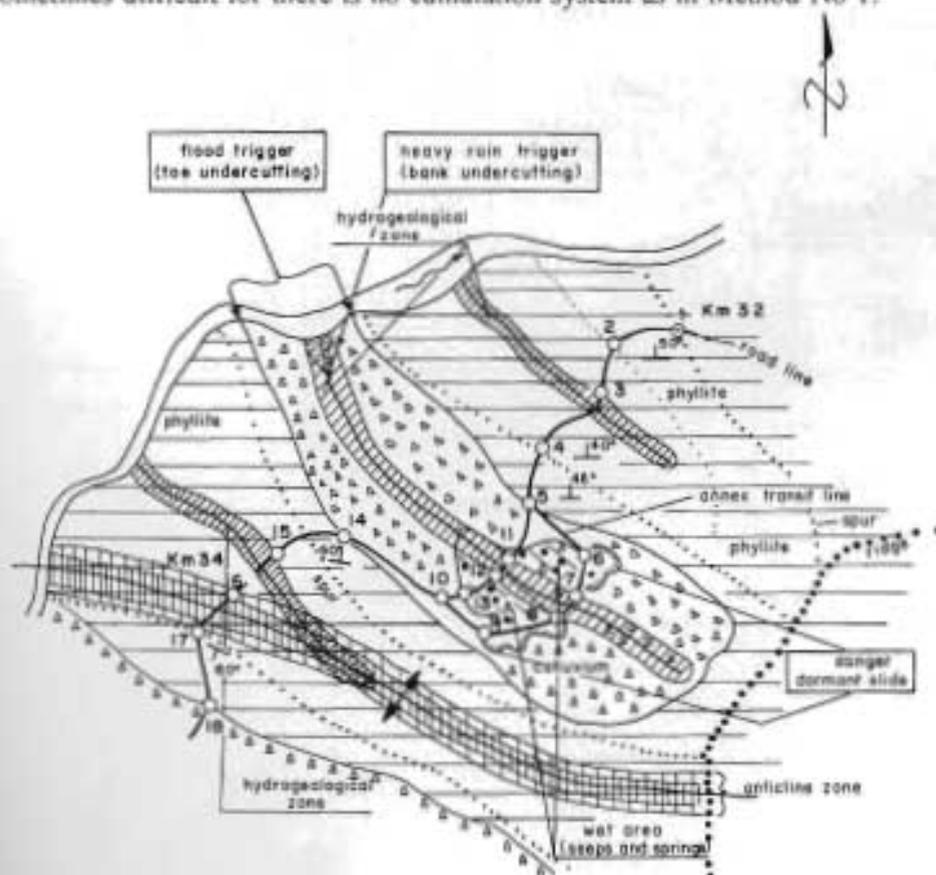
Figure 23.20 Method of surveying for hazard maps
