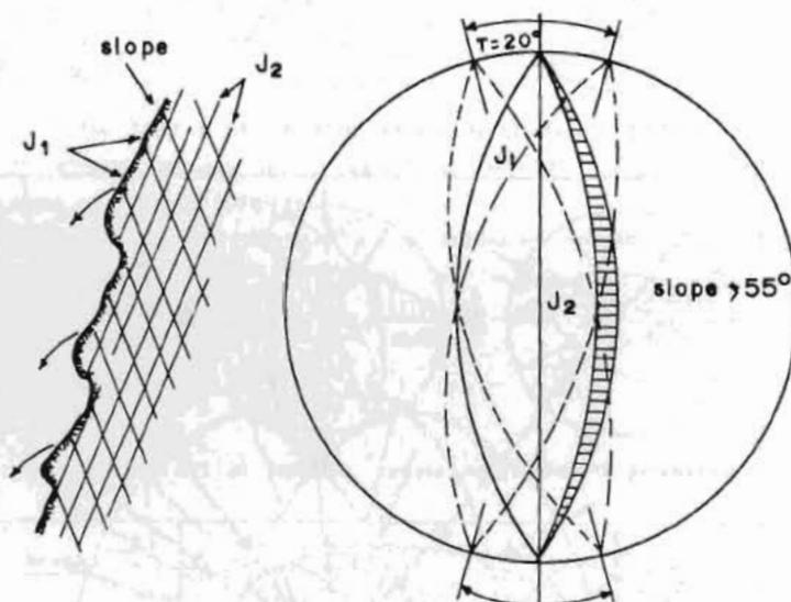
**Fig. 23.12** Structural conditions necessary to rock topple,  $t =$  strike F1 and tolerance angle F2
