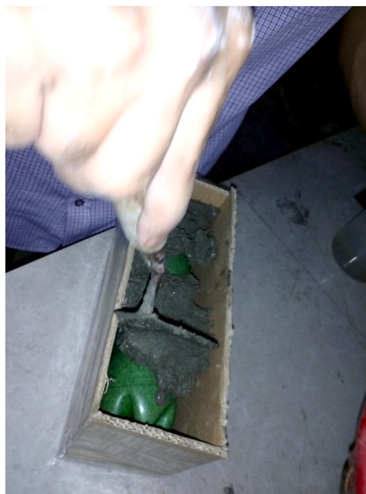
Fig. 7. Preparing a plastic brick sample with blended mortar cast in the cardboard frame and the PET plastic bottle set in the center.
