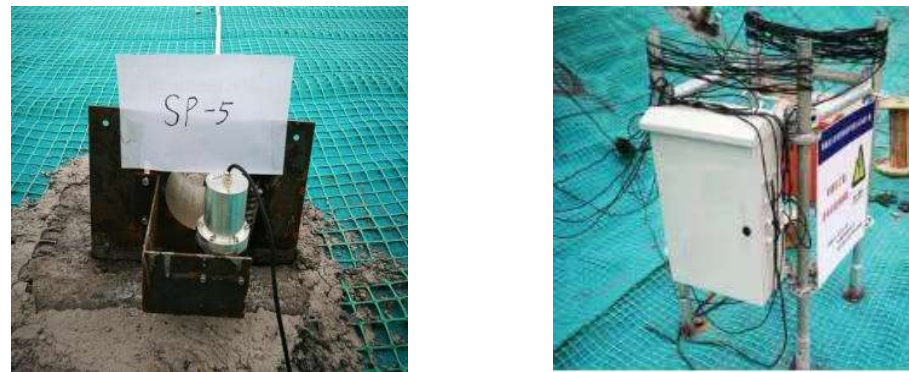
Figure 11. Pull-wire displacement sensor and station.
