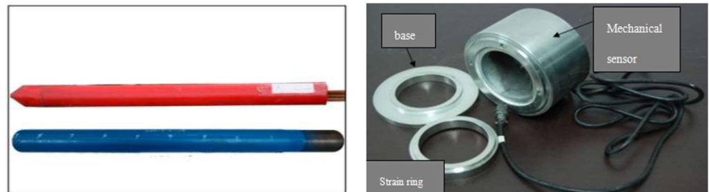
Figure 3. Sensors for measuring force and deformation.
