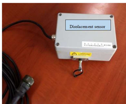
Figure 2. High-precision and large-range cable displacement sensor.
