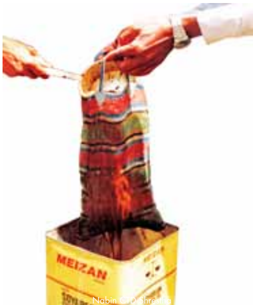
Step 4: Filtering the melted wax through a cloth bag
