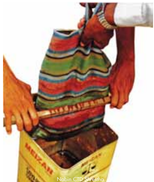
Step 5: Squeezing the bag with two sticks to extract the remaining wax
