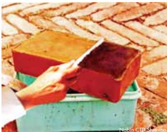
Step 6: Scraping the sediment from the base of the solid wax block
