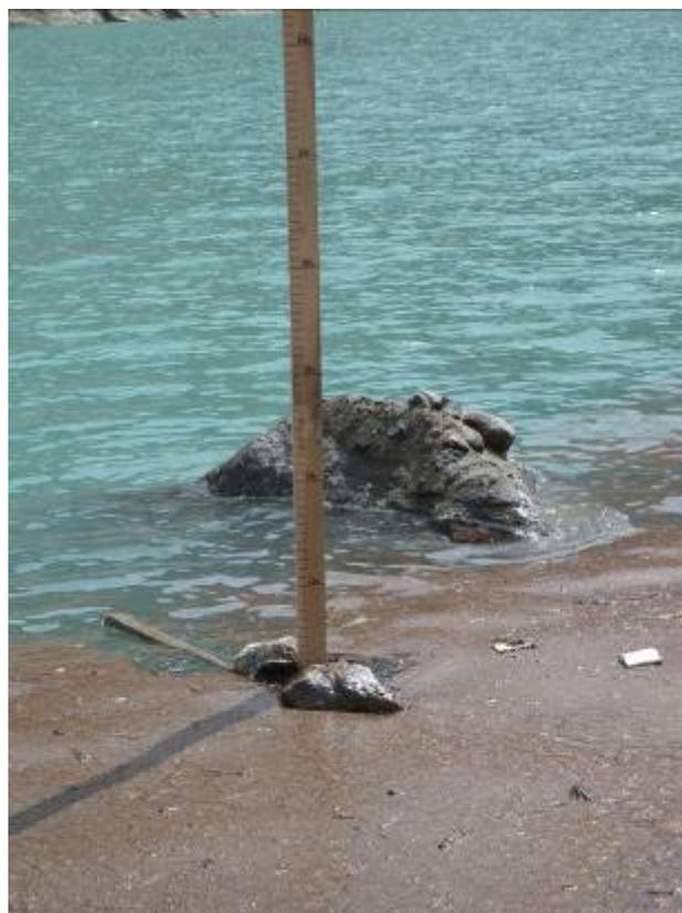
Figure 13: Hydrometric pole.
