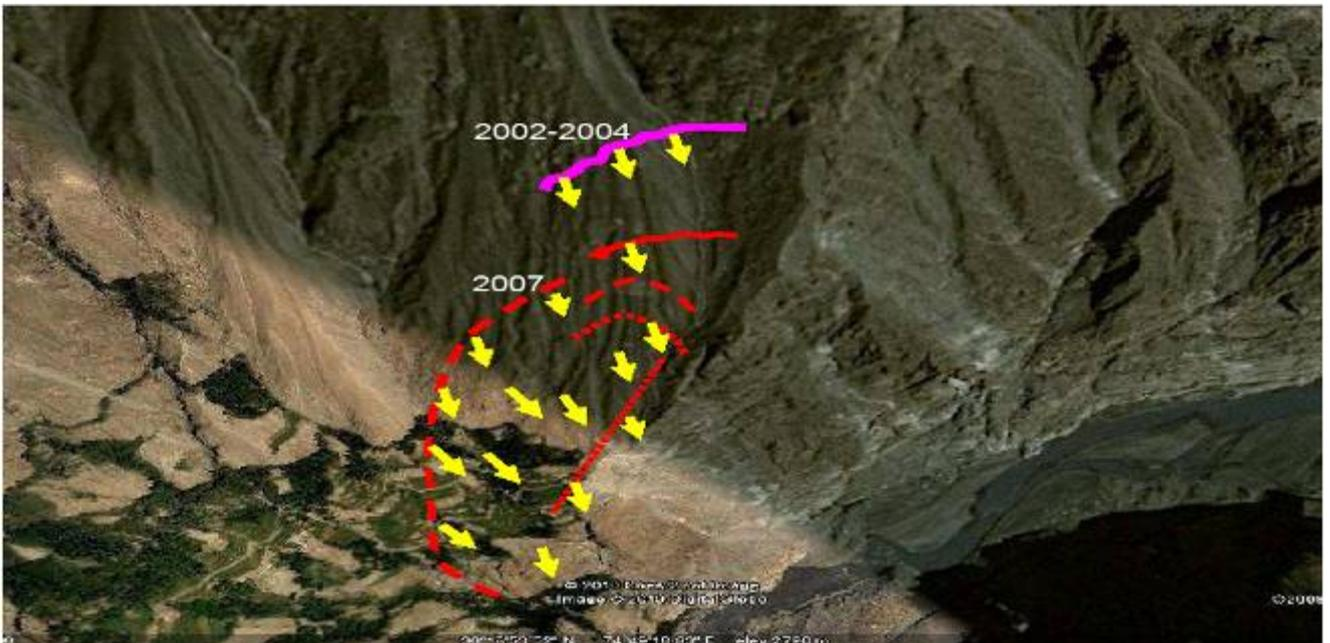
Figure 5: The main scarp of debris on the slope in 2002-2004 and 2007 at Attabad (Karim. E, 2002 Focus Humanitarian Assistance).
