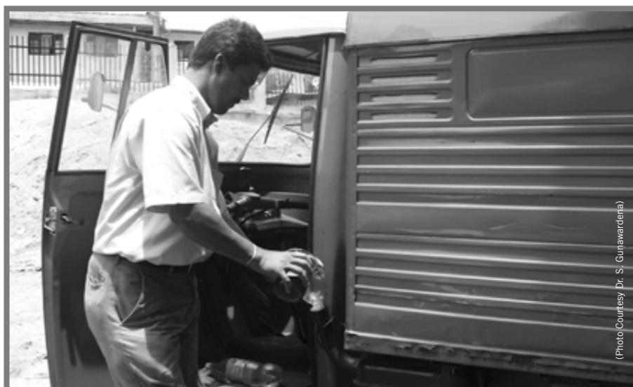
Three wheeler powered by biodiesel from neem seed oil, produced by the Department of Chemical and Process Engineering, University of Moratuwa
