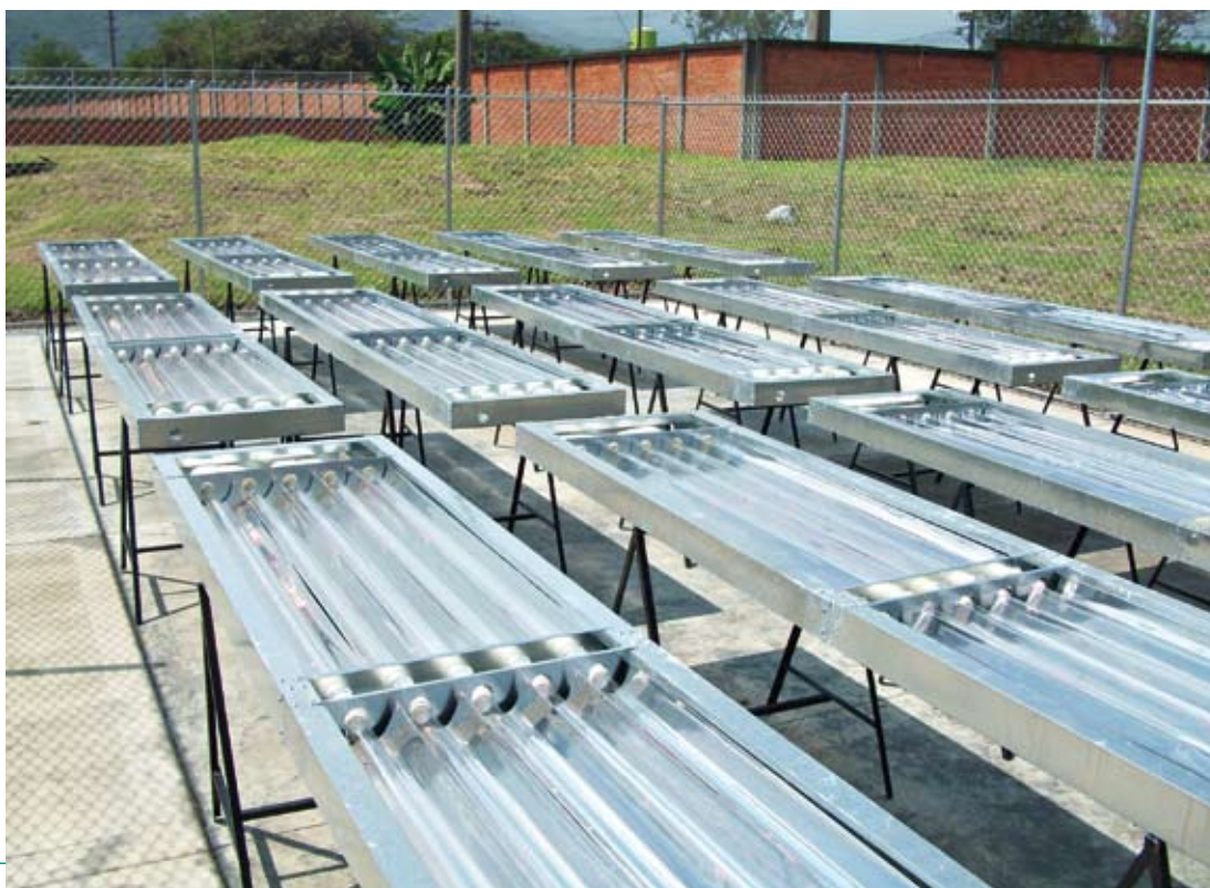
Solar reactor for bleaching wastewater from an industrial paper mill
