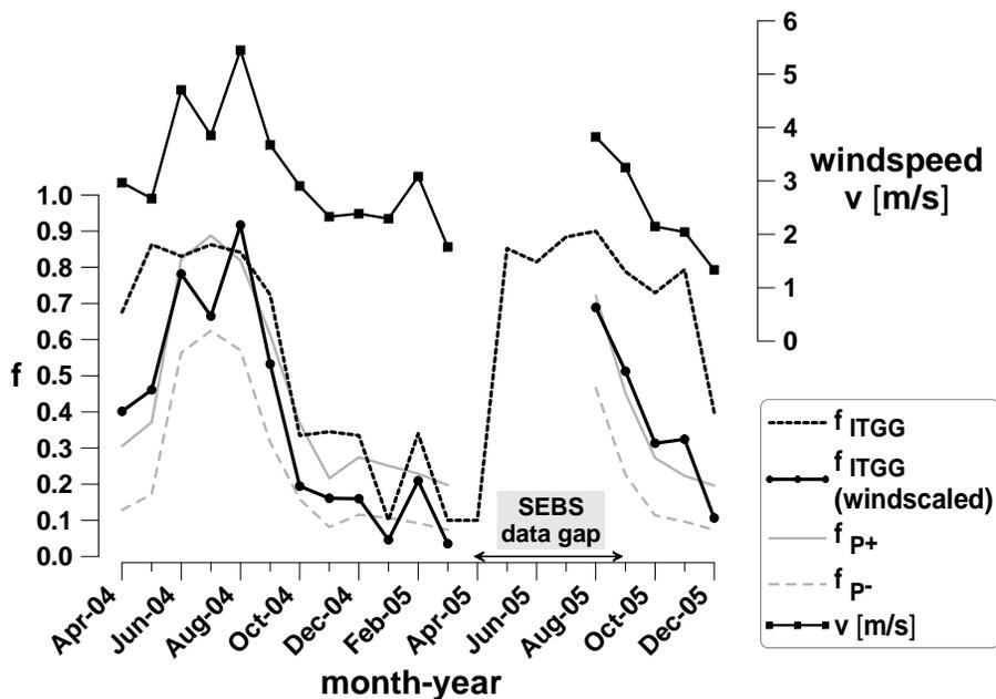
**Fig. 5.** Differently determined monthly values of  $f$  between April 2004 and December 2005. The uppermost graph refers to the right y-axis and shows the mean monthly wind speed ( $v$ ), measured at the SEBS.
