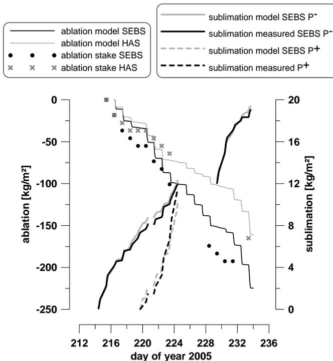
**Fig. 4.** Measured and modelled cumulative sublimation and ablation for the SEBS and the HAS. The gaps of the sublimation records refer to the gaps of the measurement series. Therefore, the sublimation values do not represent the actual sum of sublimated mass during the respective period. Note the different axis scaling, which was chosen to balance the figure graphically.
