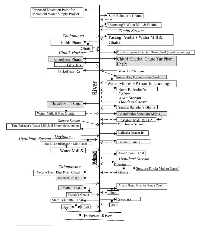
*Explanatory Note*: Ghatta - Traditional water mill used for milling grains; Water Mill - Improved turbine type water mill used for several purposes including milling/grinding of grains; IP – Irrigation Project; (P) – Planned; (O) – Ongoing ; HP – Hydro Power.
