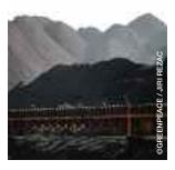
image Conveyor belt and stockpiles of coal unloaded from bulk carriers.
