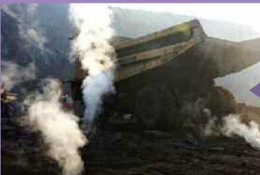
A loading truck at the Rajapur Mining Project. Smoke and noxious fumes from the underground coal fires escape into the atmosphere. Smoke from the fires contains poisonous gases including carbon monoxide, carbon dioxide, sulphur dioxide and nitrogen oxide.
