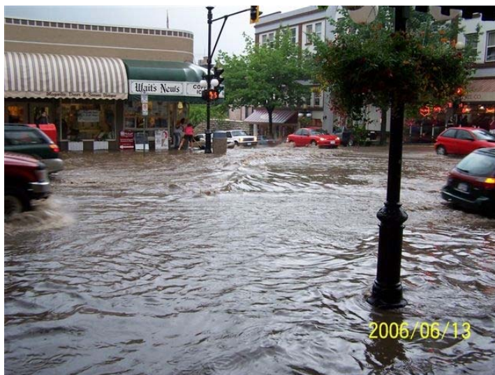
Heavy rains on Baker St in Nelson, BC, 2006 resulted in water running off the pavement and into the sewer systems. Increasing volume and pressure overwhelmed the underground piping and burst through manholes along several streets and some sanitary lines including toilets without check valves.
