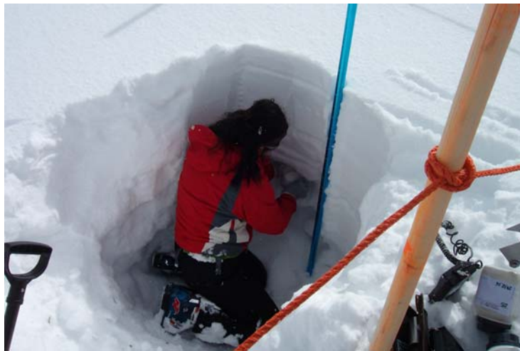
Fig. 1 - Sampling snow layer for pH and conductivity determination in Arabba site, Dolomites, Italy. Photo: M. Pecci
