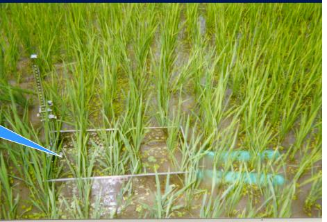
A weir system was set up at three positions on the paddy bunds (7 weirs at each position, totaling 21 weirs
