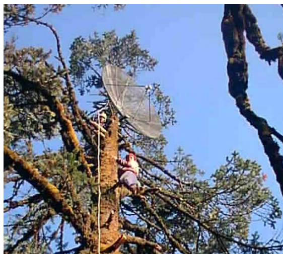
The first long range testing from Mohare to Pokhara (34 KM) putting dishes on the tree
