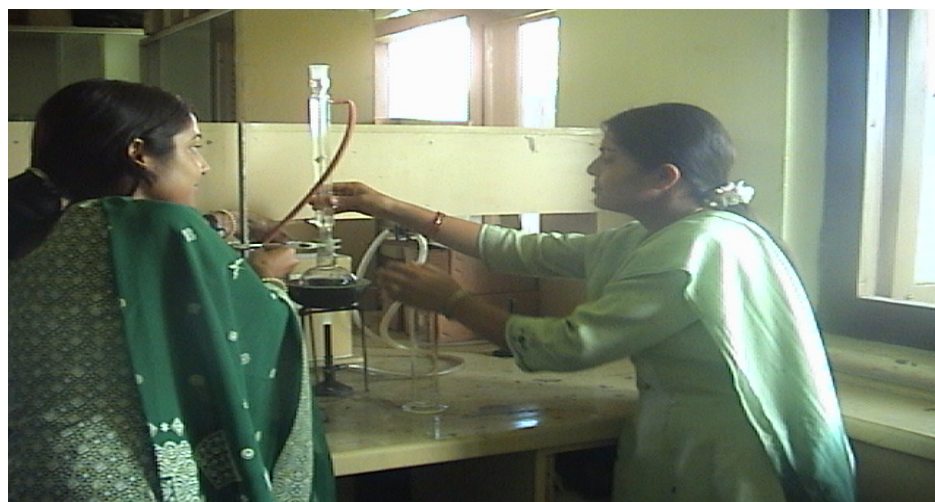
Figure 4: Setting for COD refluxing.
