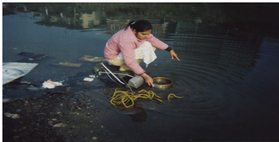
Figure 3: Washing the sediments with benthic macroinvertebrates to remove clay.
