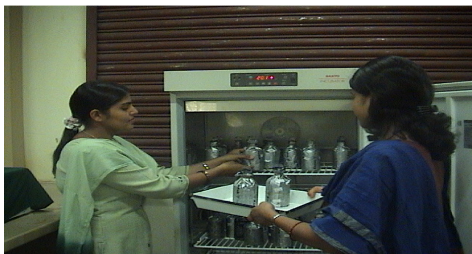
Figure 5: Putting BOD bottles inside BOD incubator.
