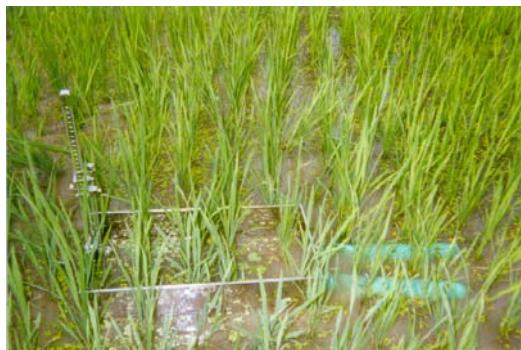
**Figure 2: Lysimeters were installed in the paddy field**
