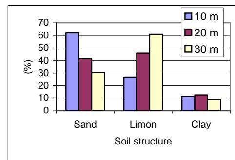
**Figure 10: Effect of sedimentation on distribution of soil texture at different distances from the base of upstream discharge inlet into the paddy fields.**
