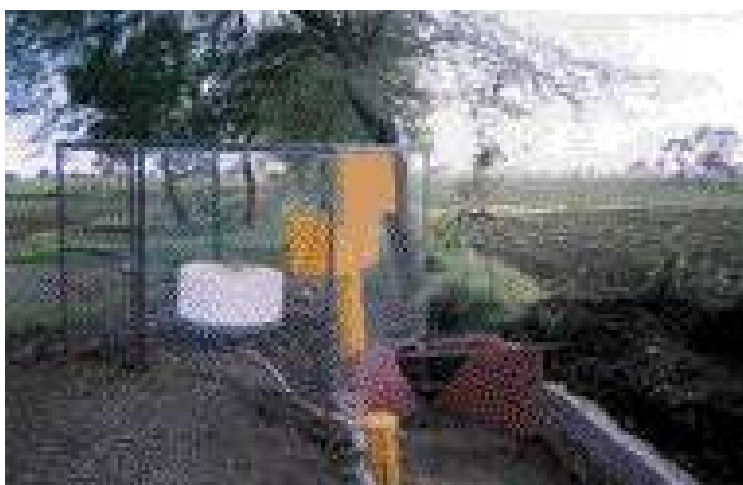
Figure 3.6. The runoff and sediment sampler used for measuring runoff and soil loss installed at Ringnodia watershed.
